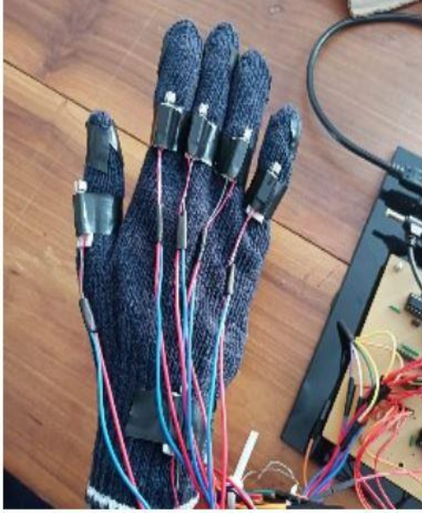
Braille Gloves to assist visual and hearing-impaired people for communication and learning.
